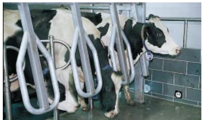
The open bottom neck rail design promotes free cow flow allowing a cow to enter the stalls naturally with her head down. This reduces load time and increases throughput.
